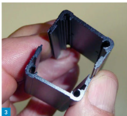
Fig. 7: Front with aperture cut out and holes drilled.
